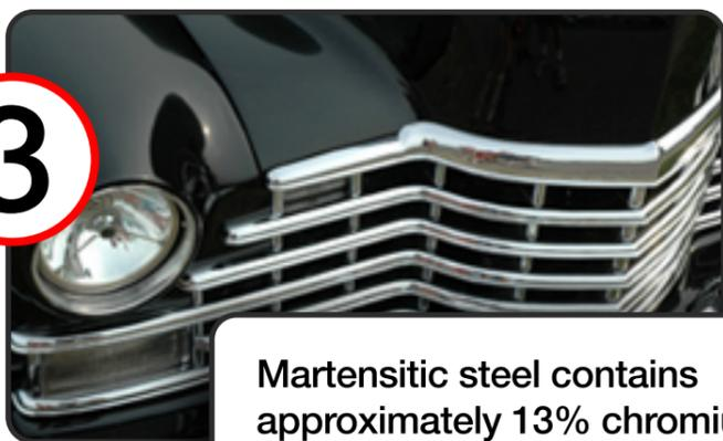
Martensitic steel contains approximately 13% chromium. Type 410 is a widely used, low-cost, general purpose steel used for applications where corrosion potential is moderate.
