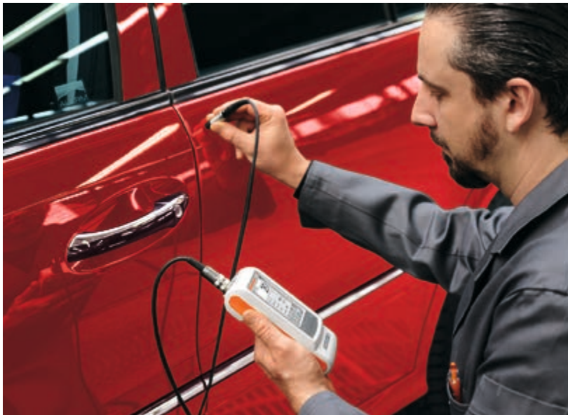
Measurement of auto body paint thickness using the dual probe FD13H
