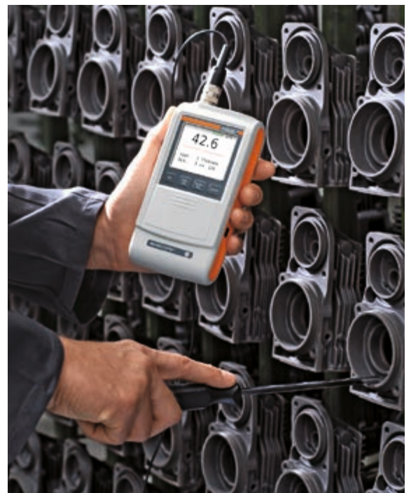
Measurements using the internal probe FAI 3.3-150
