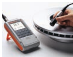
DELTASCOPE® FMP30 using dual-tip probe V7FKB4
