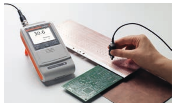
ISOSCOPE® FMP10 using the probe FTA3.3-Cu
