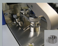
Adapter for wires with a diameter of 1-3 mm
