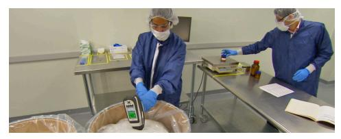
The analyzer can measure directly through plastic drum liners and glass containers permitting analysis without opening the packaging.
